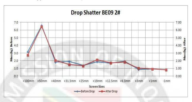
The blasted 2A seam had a percentage -0.81mm of 3.64% (m/m) which was similar to the drop shutter test results on the -0.81mm of 3.6% (m/m). The stability of the blasted 2A seam BE09 coal was 1.01 with a friability of 98.991%.
