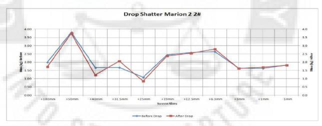
The freely digged 2 seam had a percentage -0.81mm of 7.91% (m/m) which was very close to the drop shutter test results on the -0.81mm of 8.1% (m/m). The stability of the freely digged 2 seam Marion 2 coal was 1.0 with a friability of 98.999%.
